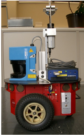
Figure 1: Robot platform Pioneer 3DX equipped with Microspace PC and omnidirectional camera
