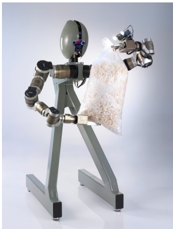
Fig. 1: The dual-arm manipulator with the static frame
