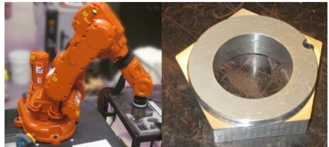
Fig. 5. An ABB IRB-140 industrial robotic arm (left) was configured to assemble an aluminum pentagonal puzzle insert (right).
